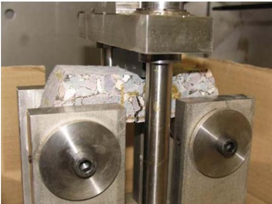
Figure 4: Set up 3-point bending test.
