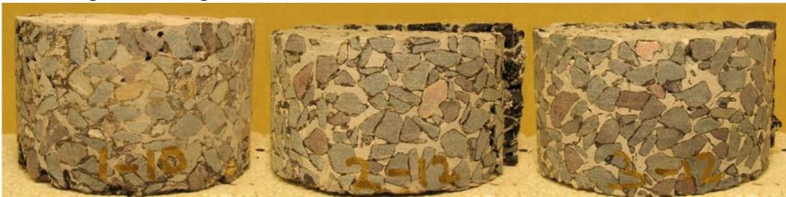
Figure 2: Detailed sections grouted macadam (1: B70/100; 2: 4.3% PMB; 3: 4.7% PMB).
