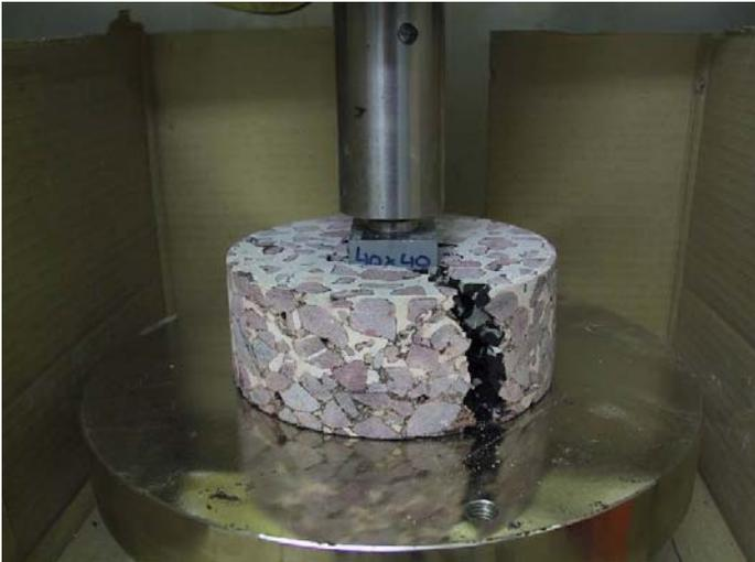
Figure 3: Set up Stebocon indentation test.
