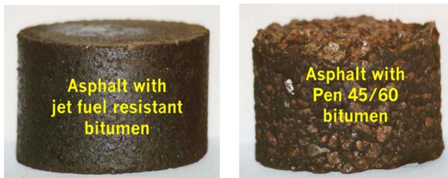
Figure 9 Marshall specimens after 24 hours immersion in jet fuel
